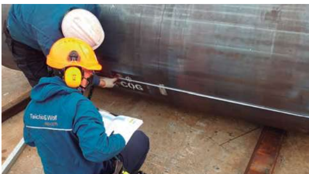
Dimension Control Inspection
