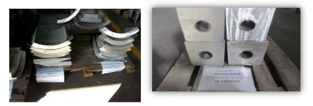
One anode per each type will be sectioned during the PQT, thereafter, during production, the required number of anodes per each type will be sectioned.
