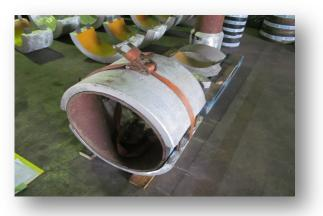
A Number of anodes per each type (as per client specification) will be assembled and fitted around a pipe in the presence of COMPANY with the same external diameter as the externally coated pipe.
