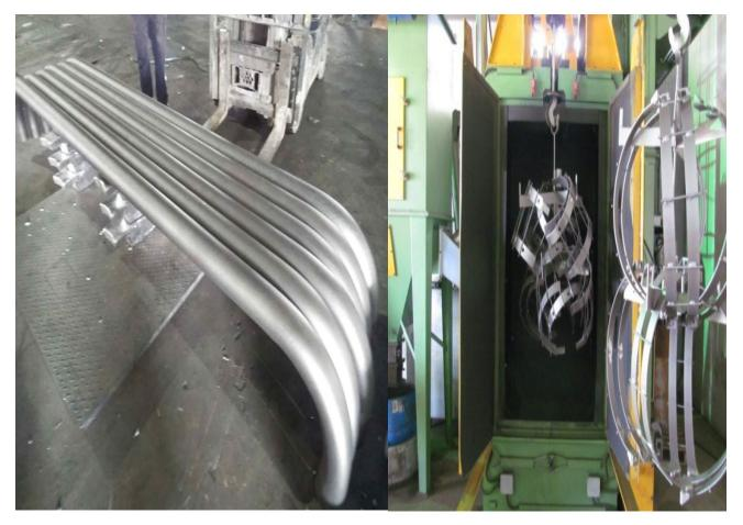
All anodes steel insert will be fabricated from low carbon steels of weldable quality with the product Carbon Equivalent value  $CE \le 0.41\%$  and carbon content C $\le 0.23\%$ .
