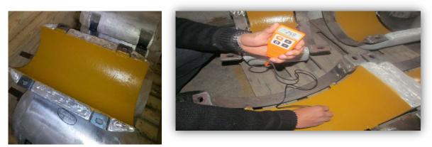
The anode underside surface (if required) is coated with epoxy paint. Coating will be as per client specification.
