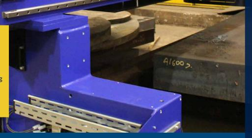
The machine offers Oxy Gas cutting and while one of the oldest processing options within the industry, it is as popular as ever. With the ability to cut through 450mm thick pieces of steel in a timely manner, Oxy Gas cutting offers a reliable and fast service with 6 cutting heads speeding up processing time. The addition of drilling, enables fast turnaround of finished parts to industry standards.
